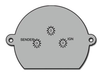
Make sure you connect wire to terminal as marked. Sender to Sender and IGN to power Nothing will be connected to screw in upper center position
