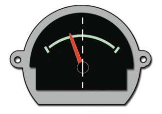
When Vehicles is running at 160° or 180° the needle of the temperature gauge will be pointing approximately 1/8" left of center point as shown.
