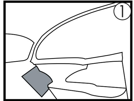
**\*\*\*TMI Products Rear quater panels must be installed prior to installation of TMI Products complete rear seat\*\*\***
