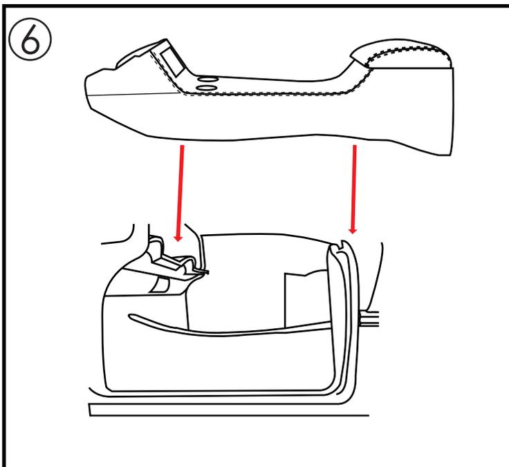
**Step 6:** after the fiber glass has been cut you can now Re-Install your shifter linkage. You will put the TMI Products center console over your shift linkage. Then with the center console in you will stick your shifter through the console and attach it to the linkage. Then slide the shift boot down the shifter into place on the console. Installing your shift knob last. View page 1 step 2 for final step.
