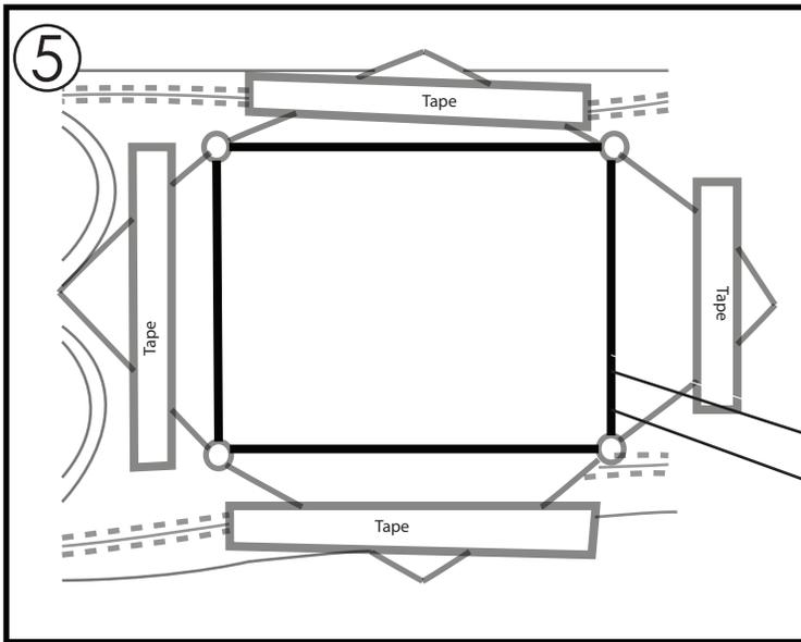
**Step 5:** Once you have pulled back the vinyl you will need to cut the fiber glass. The best way to do this is to use a cut off wheel to cut at all four corners where your guide holes should be drilled you will cut from each guide hole to the other.
