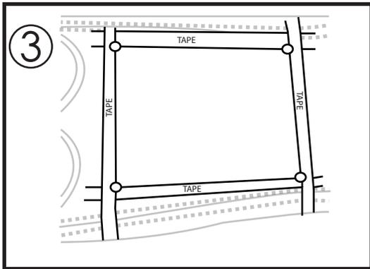
**Step 3:** Next you will need to drill guide holes. using your masking tape lines drill holes at the corner of your measurment. Start with a 1/8th inch bit the go up to a 1/4 inch bit. Hold the vinyl at each side so the drill bit does not pull the vinyl from the fiberglass.
