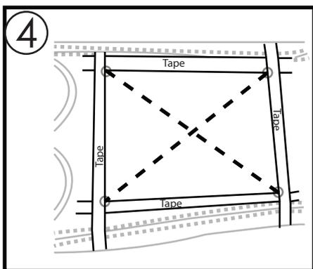
**Step 4:** Once the guide holes are drilled, cut an "X" on the vinyl to each guide hole so you can peel the vinyl back and tape each vinyl triangle into place reveling the fiber glass
