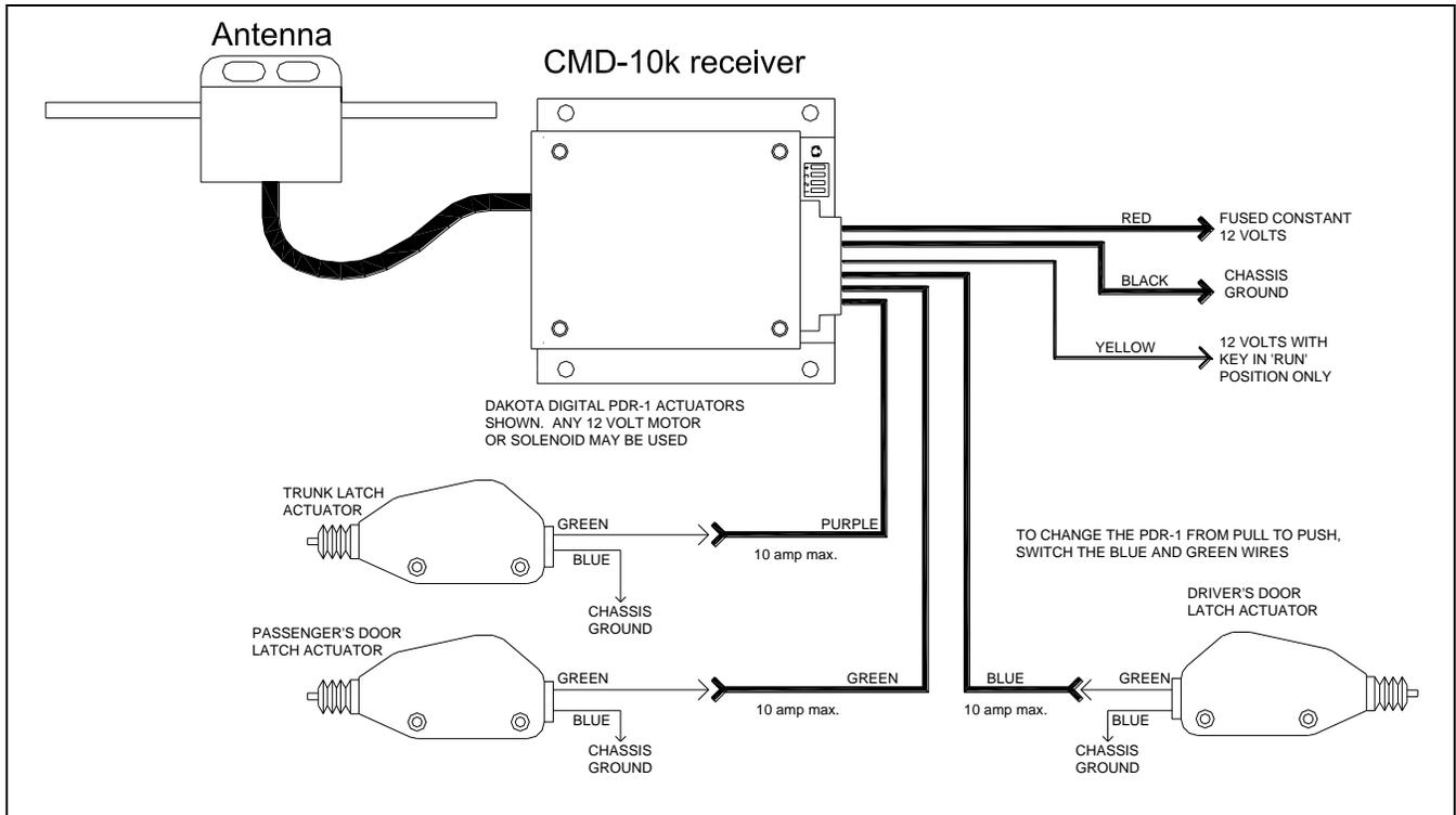
Figure 1. Door and trunk latch wiring diagram.
