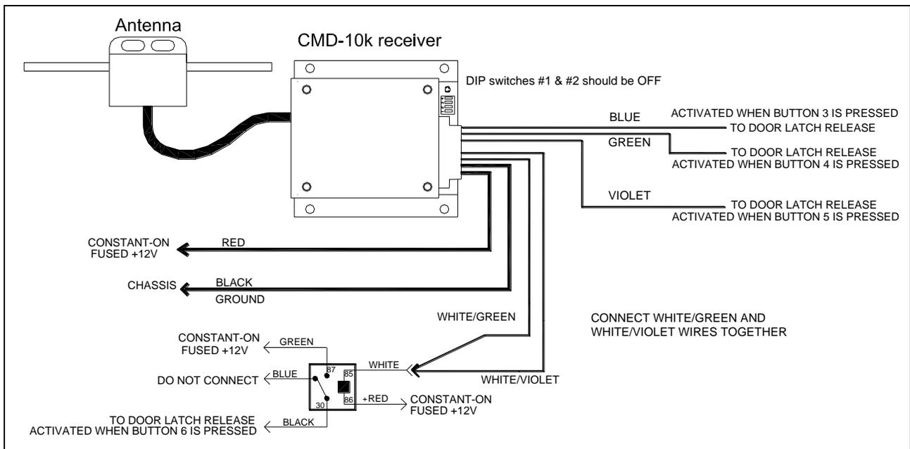
Figure 12. Connection for operating four door latch releases.
