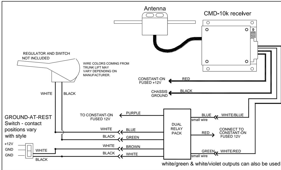
Figure 7. Connection to power trunk lift motor.
