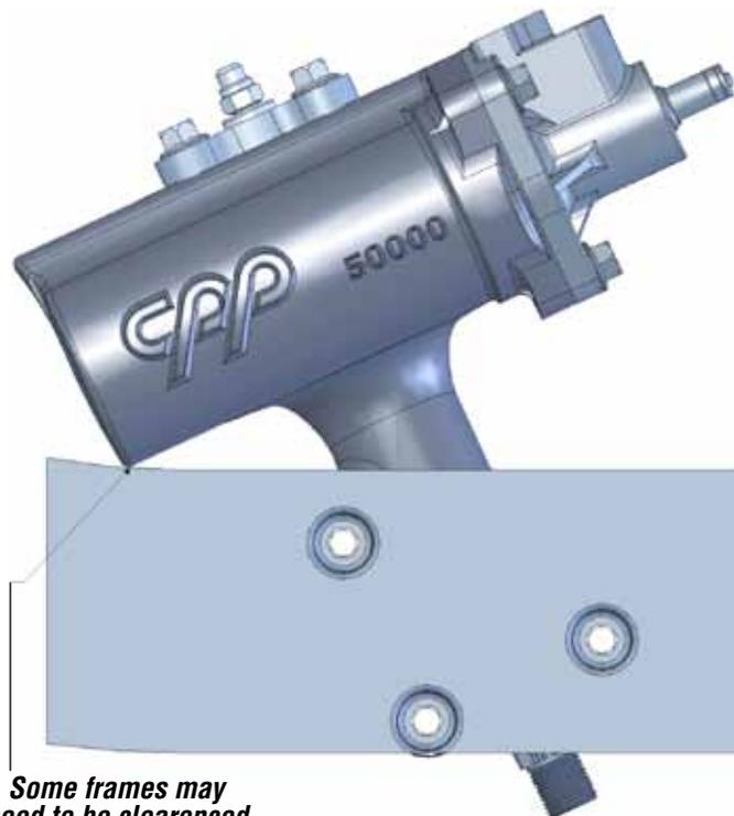
**Some frames may need to be cleared here. Do not grind on the steering box!**
