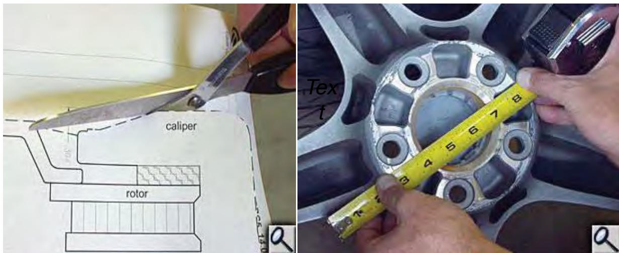
After you have cut the template along the bold dotted line, measure the inside diameter of the wheel where the hub goes inside the wheel. The wheel in this photo has a chamfer at the top of the hub hole.
