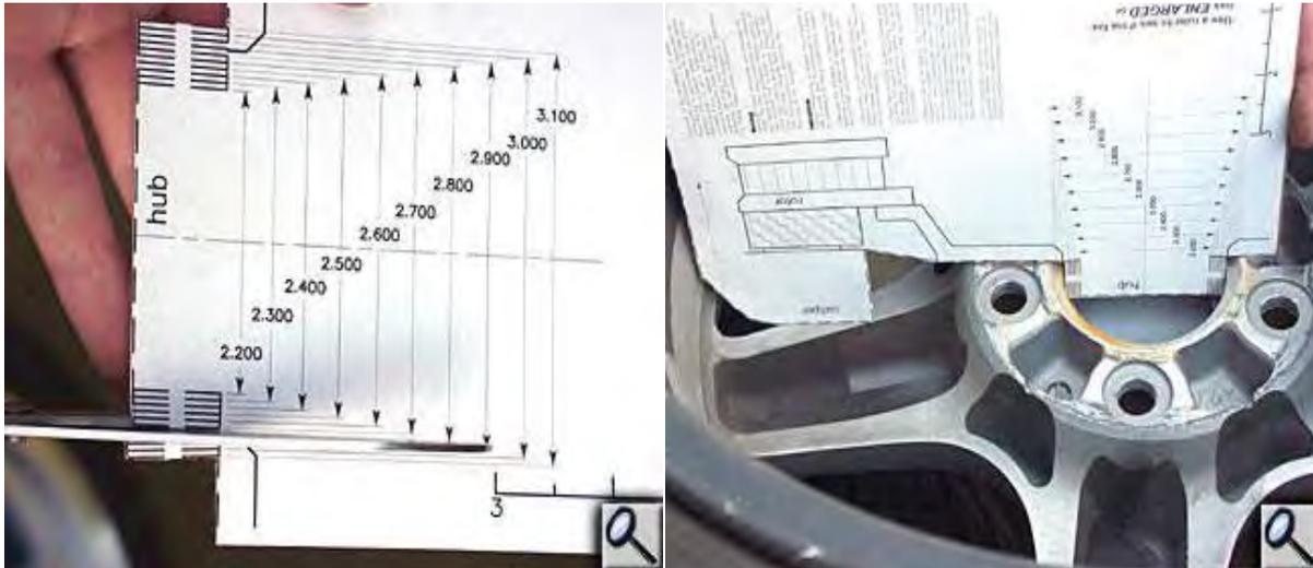
Once you have trimmed the hub area of the template, place the template into the back of the wheel. The hub area of the template should fit down into the hub hole in the wheel. This "Extreme" system template fits into this wheel with one exception; the template is resting on the spoke of the wheel and not allowing the template to rest flat on the hub section of the wheel. Also note that the template is very close to hitting at the top of the wheel to the top of the caliper.
