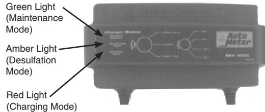
**NOTE:** The Battery Extender may switch back into full charge mode (Red light ON) as required by your battery, this is normal.
