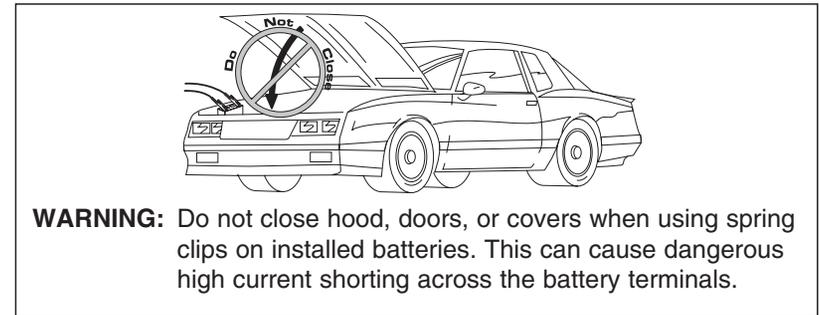
1. Check that the Battery Extender is **NOT** plugged in to an AC outlet before connecting the spring clips to the battery.
