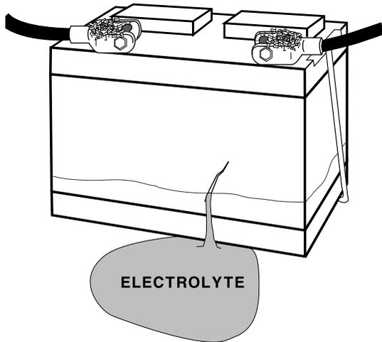
■ **Important Note:** A damaged battery must be replaced before proceeding.
