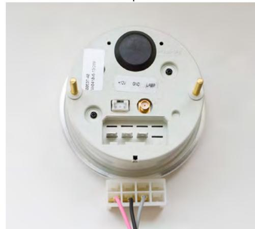
You may remove or simply not connect the purple wire when using a GPS Speedometer. Electric Speedometers that use an interface module still require the purple wire.
