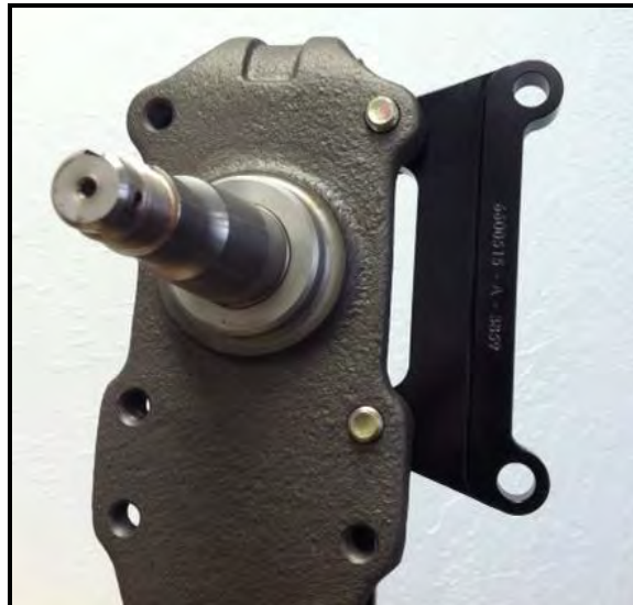
Figure 2: Base bracket installed onto spindle
