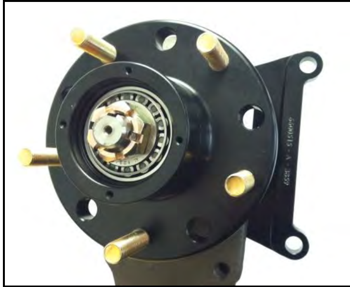
Figure 3: Hub installed onto spindle
