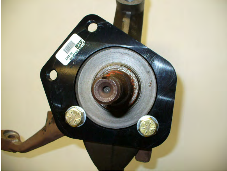
Spindle bracket mounting for Rear Steer applications
