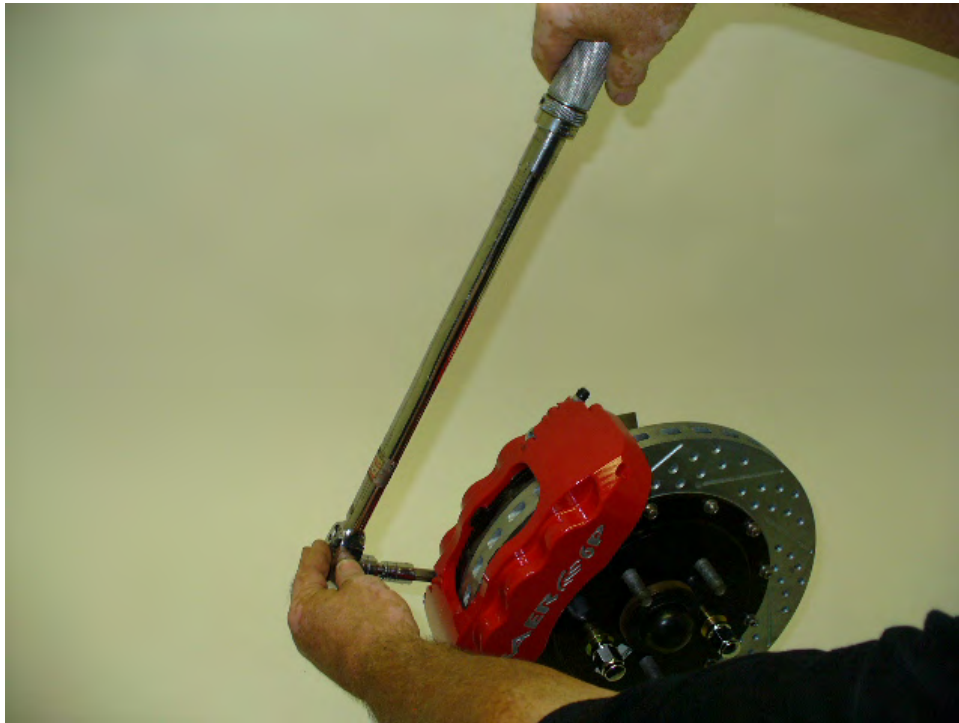
Torque caliper bolts to 85 ft-lbs.
