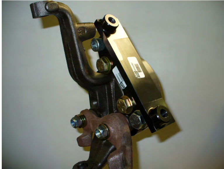
Radial mount bracket installed.
