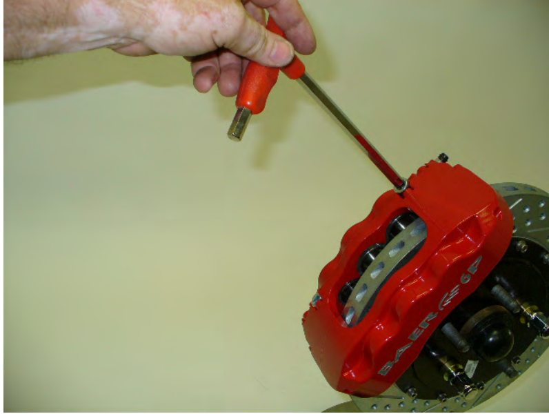
Install the caliper to measure clearance.
