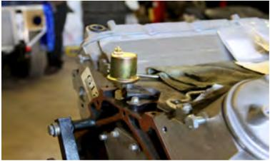
**Oil Temperature:** All of the previous with oil pressure applies as long as you use an electric gauge. There is room (especially if you plan ahead) to install an oil pressure, and 1/8"npt oil temperature port on the same cover plate. Using a mechanical oil temperature in this location is not recommended due to the size of the probe requiring a minimum 3/8"npt (with a 2263 adapter), which measures nearly 5/8" in diameter.
