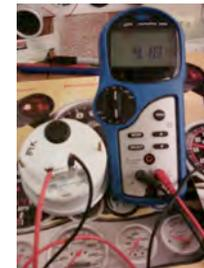
If you get a measurement of 2.9K, you may then send the speedometer into us for service to have an internal circuit modification performed. This modification in most cases will remedy the problem. If you get a measurement of 4.6K or higher, then no modification is needed.
