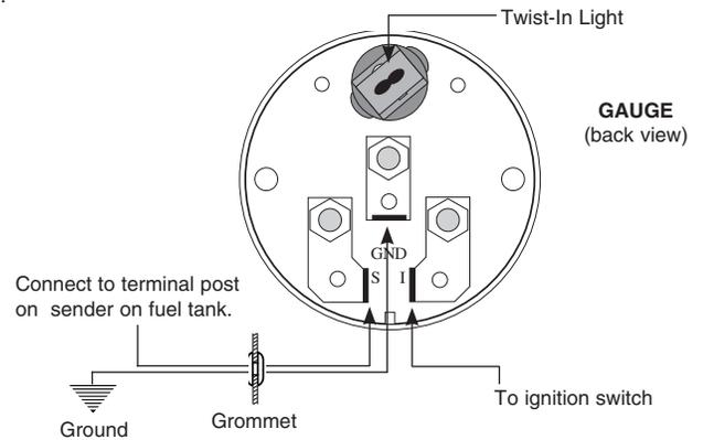
**INOTE:** Failure to ground sender as in step 5 may result in inoperable gauge.
