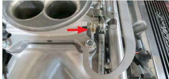
c. Using a timing light, adjust the distributor to 12° BTDC. Then tighten down the distributor clamp.
