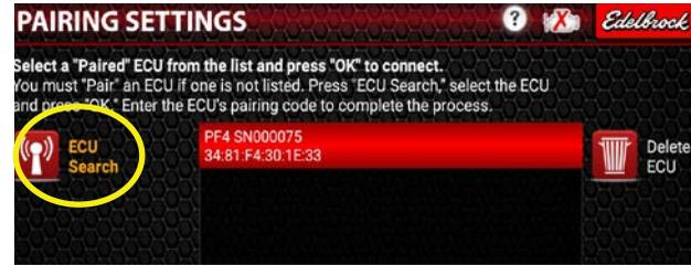
7. The title bar across the top of the screen will flash yellow, indicating that the device is attempting to communicate with the ECU. Once E-Tuner connects to the ECU, it will proceed to the Setup Wizard start screen. Proceed to Step 8.
