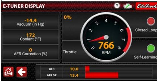
**Digital Display** - A numeric display for monitoring all parameters used by the Pro-Flo 4 System.
