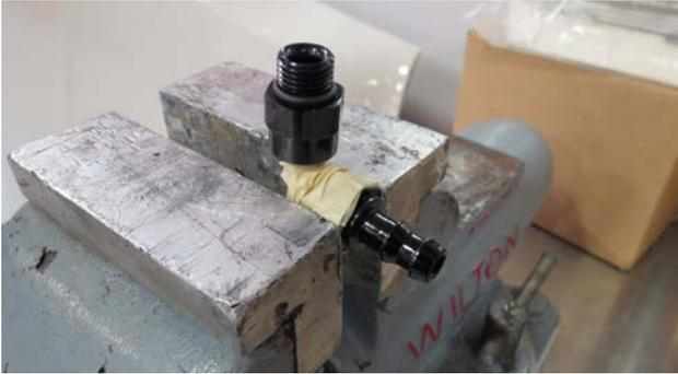
2. Lubricate the barbed end on the fitting with silicone lube as well as the inside of the hose end that will mate with the fitting.
