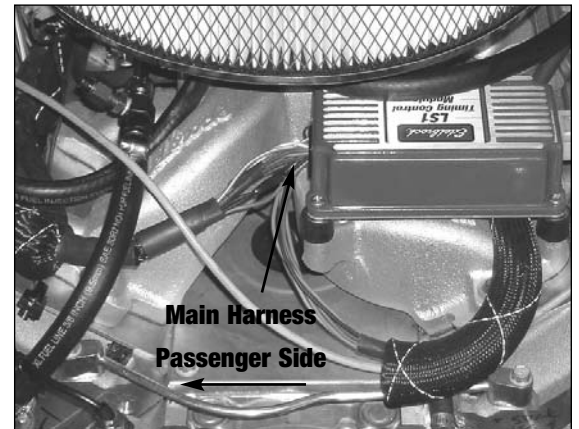
Figure 4 - Timing Control Module Mounting
