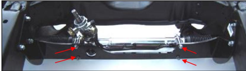
When mocking up the shaft, if you need extra clearance, you can rotate the rack & pinion on the bracket about 10°. Loosen the nuts of the two U-Bolts holding the rack & pinion to the bracket, rotate, and then retighten. **Torque to 18 ft/lbs. Do not overtighten.**
