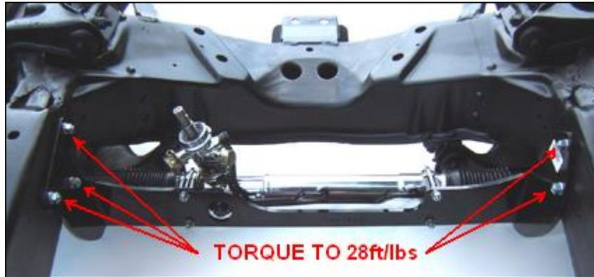
Line up the holes in the mounting brackets to the holes in the frame, where the steering box and idler arm were. Bolt brackets onto the frame, using mounting hardware kit #620340. Nuts to the inside of the frame, bolt the brackets into the frame with 28 ft/lbs of torque(see illustration Above).
