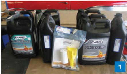
The key to setting up your cooling system for waterless coolant is getting as much water out of the system as possible. When you have completed the installation you are going to want only 3% or less of water. Any more and the effectiveness decreases drastically. Using the Evans Coolant Conversion Kit and the Prep Fluid you should be able to hit this number with no problems, but we will tell you what to do if you don't. Let's get started.
