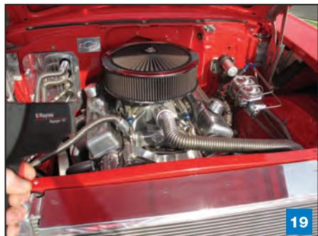
9.) Once the engine is cooled off completely we need to drain all the Prep Fluid from the radiator and engine block. Repeat steps 1 thru 5 above to do this. You can save the Prep Fluid in the original containers for reuse up to 3 times. Just be sure to keep the containers closed tightly. Get as much of the Prep Fluid out of the system as possible. The little that will be left is compatible with the Waterless Coolant and will do no harm.
