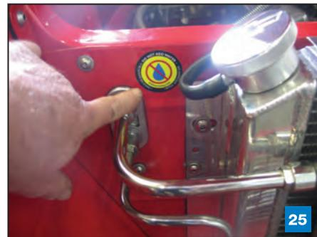
That's pretty much it. The Evans system isn't cheap, but as it protects so much better (-40° to 375° F), helps your radiator, heater core, heater control valve and water pump last longer, prevents corrosion and basically lasts the life of the vehicle it is well worth the effort and expense in our book. You will want to check it periodically to be sure the water concentration is below 3% but other than that you don't have to do anything with the coolant ever again.
