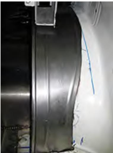
011- Final Fit. Final fit and trim. Remove paint for the welding next.
